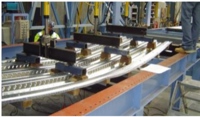
Formwork – Point Load
